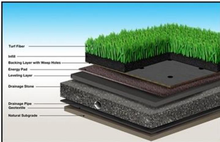
Figure 1. Anatomy of Artificial Turf
